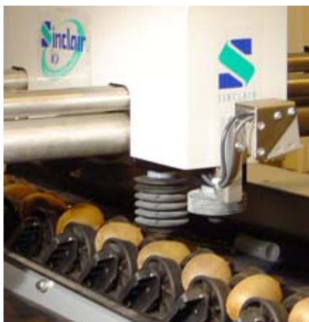
The Sinclair iQ firmness tester, a non-destructive high speed system for measuring the firmness of individual fruit on-line.
