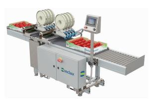
Perfect for labeling fruits and vegetables in inners or trays, this is a two-arm model with seven-inch touchscreen interface, automated lift arms, remote access capability and user-friendly controls that complement a state-of-the-art packinghouse operation. This system can label up to 16 rows of fruits and vegetables in one pass.
